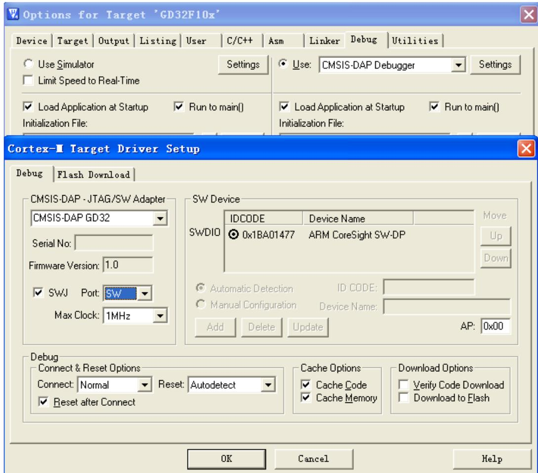
Select "Utilities" page, and then select "CMSIS-DAP Debugger", then click "Settings" command button, "Add" the correct flash programming algorithm according to the GD32 MCU which is using.
