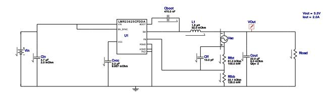
1. The input capacitor included in the BOM only contains a small filter capacitor that should be placed near the IC. Depending on where the power supply is laid out in the system additional bulk capacitance may need to be added to filter the line ripple.
